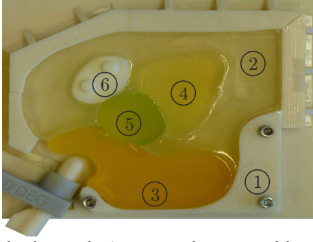
Fig. 2. The phantom that incorporates the anatomy of the male pelvic region. The anatomy is coloured for clarity. ①: Spine, ②: Adipose tissue (fat), ③: Rectal wall, ④: Urinary bladder, ⑤: Prostate and ⑥: Pubic bone.
