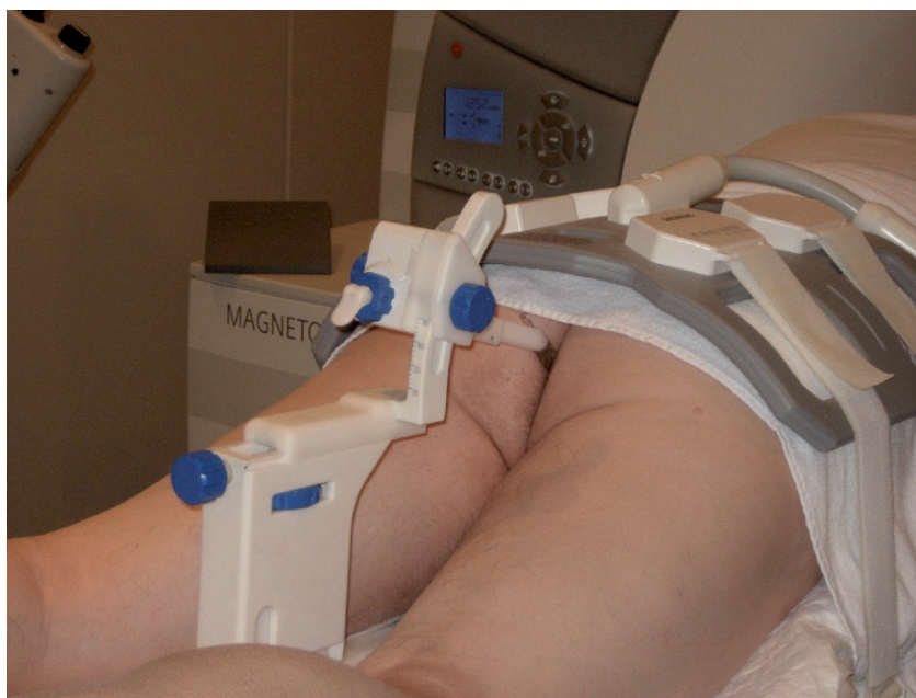
Figure 1. Magnetic resonance-compatible mechanical positioning device. Reproduced from [46].
