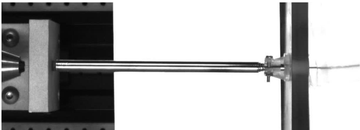
Figure 33. A 0,8 mm needle with a bevel angle of 45° inserted into a 20% gel at  $5 \text{ mm s}^{-1}$  with sheath
