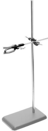
Figure 17. Ultrasound head placement device.
