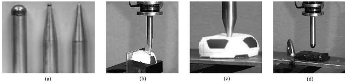
**Figure 6.** (a) Tools tested and measuring tool-material interaction forces during (b) and (c) deformation of rubber and (d) deformation of bovine liver (Mahvash et al., 2002). Images printed with permission from publisher (EuroHaptics 2002).
