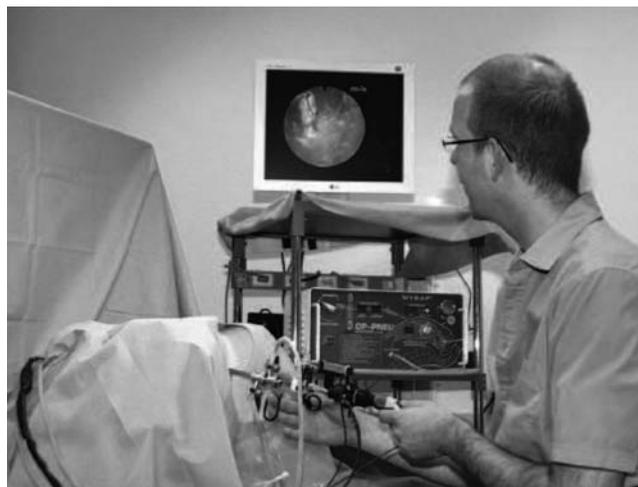
**Figure 1.** Hysteroscopy training simulation environment coupled with a haptic device (Harders et al., 2006). Reprinted from *Studies in Health Technology and Informatics*, Vol. 119, Harders et al. *Highly realistic, immersive training environment for hysteroscopy*, pp. 176–181, ©(2006), with permission from IOS Press.
