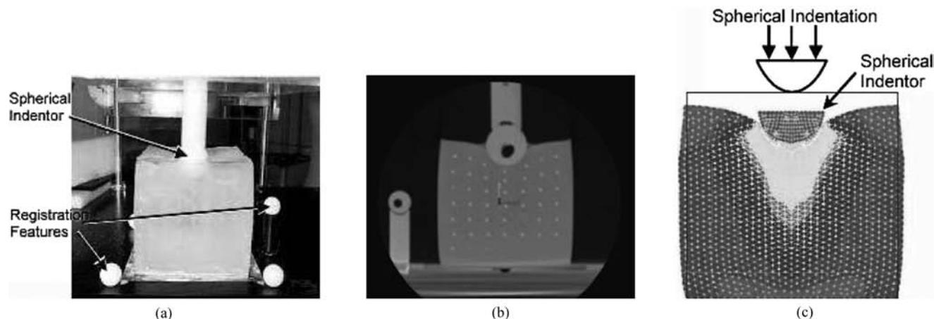
**Figure 7.** Indentation test on the “Truth Cube” embedded with fiducials; (a) experimental test setup, (b) CT of center vertical slice under 22% strain, (c) FE model under 22% strain (Kerdok et al., 2003). Images printed with permission from ©2003 Elsevier B.V.
