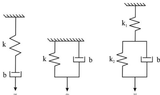
**Figure 4.** Standard viscoelastic models commonly used to represent soft tissues (a) Maxwell (b) Kelvin-Voigt (or Voigt) (c) Zener standard linear solid (or Kelvin) (Fung, 1993).
