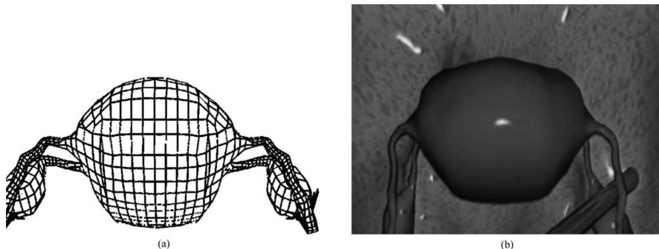
**Figure 8.** Formulation and results of the endoscopic simulator: (a) FE model of the human uterus containing 2000 elements. (b) Tool-tissue interaction model used in the surgical simulator (Székely et al., 2000). Images printed with permission from MIT Press Journals ©2000 by the Massachusetts Institute of Technology.
