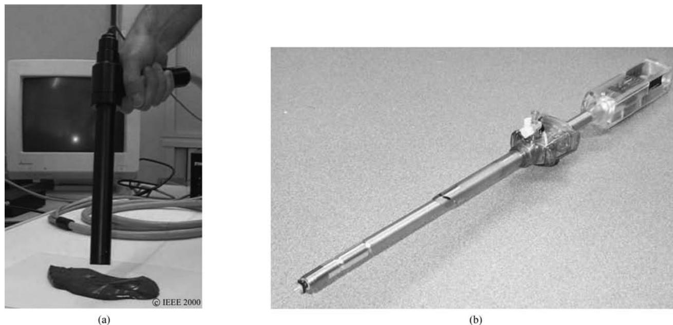
**Figure 11.** Devices used to measure tissue properties *in vivo*: (a) Tissue aspiration technique (Vuskovic et al., 2000). Image printed with permission from ©IEEE 2000. (b) TeMPeST 1-D with 12 mm surgical port (Ottensmeyer, 2002). Image printed with permission from Wiley-Blackwell Publishing Ltd.
