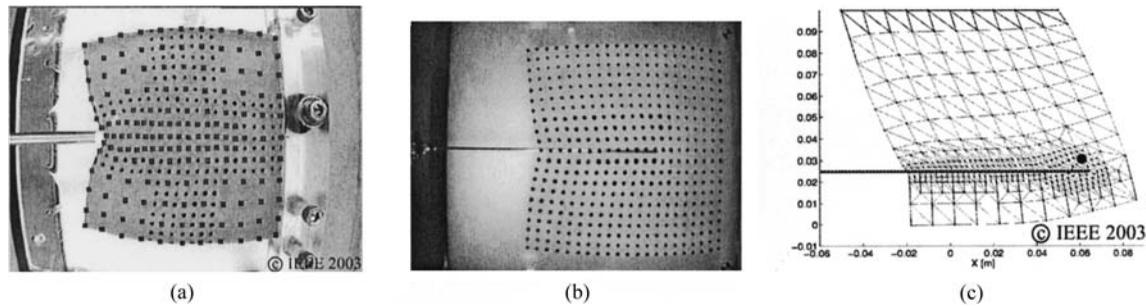
**Figure 9.** Needle insertion and simulation modeling: (a) Probing for estimation of material properties of phantom tissue. (b) 17 gauge epidural needle inserted into phantom tissue while motion of markers and insertion forces are recorded. (c) FE simulation of needle insertion with small target embedded within elastic tissue (DiMaio & Salcudean, 2003a). Images printed with permission from ©IEEE 2003.
