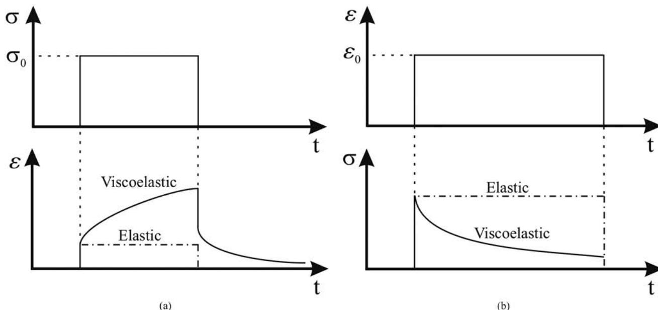
**Figure 3.** Examples of characteristic properties of viscoelastic materials: (a) creep and creep recovery—for a constant applied shear stress  $\sigma_0$  results in an increase in shear strain; (b) stress relaxation—for a constant applied shear strain  $\epsilon_0$  results in a decrease in shear stress until it reaches a steady-state value.
