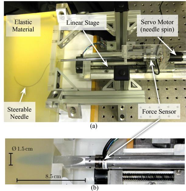
Fig. 1. (a) Experimental setup used to robotically steer a flexible bevel-tipped needle through a soft elastic material. (b) Needle with  $10^\circ$  bevel angle and  $\text{Ø} 1.5 \text{ cm}$  inserted into gel A (3:1 Plastisol gel) during the macroscopic experimental studies.
