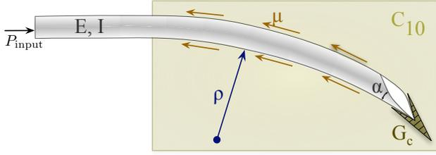
Fig. 2. Schematic of a bevel-tip needle interacting with a soft elastic medium. The two dimensional model incorporates tip forces generated by rupture, tissue properties (toughness:  $G_c$ , nonlinear elasticity:  $C_{10}$ ) and needle properties (bevel angle:  $\alpha$  and flexural rigidity:  $EI$ ).
