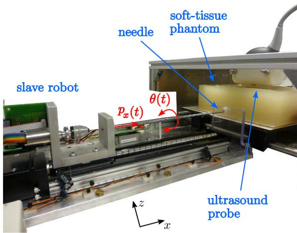
Fig. 3. Slave system. The two degrees-of-freedom robotic device steers the bevel-tipped needle according to the commanded position  $p_x(t)$  and commanded orientation  $\theta(t)$ , which come from the master device. The ultrasound probe allowed needle tracking during the insertion.
