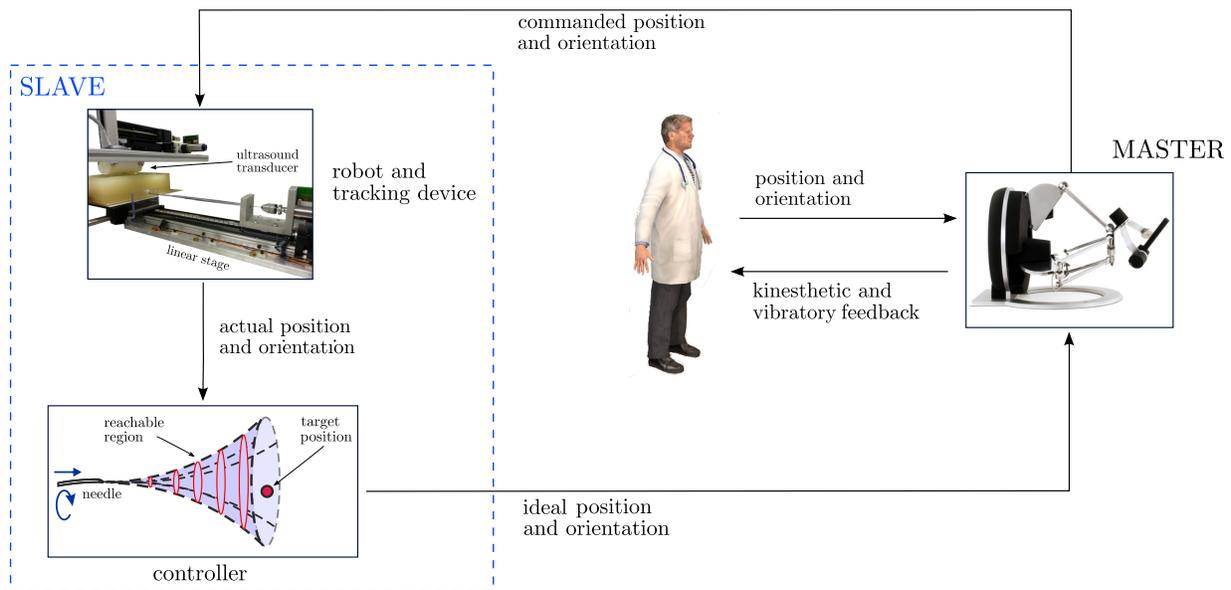
Fig. 2. Teleoperation system overview. The ultrasound-guided steering algorithm, presented in Sec. II-A, computes the *ideal* position and orientation of the needle. The haptic interface provides this information to the clinician through a mix of kinesthetic and vibratory forces, as described in Sec. II-B. The human operator then controls the motion of the slave robot from the master interface.
