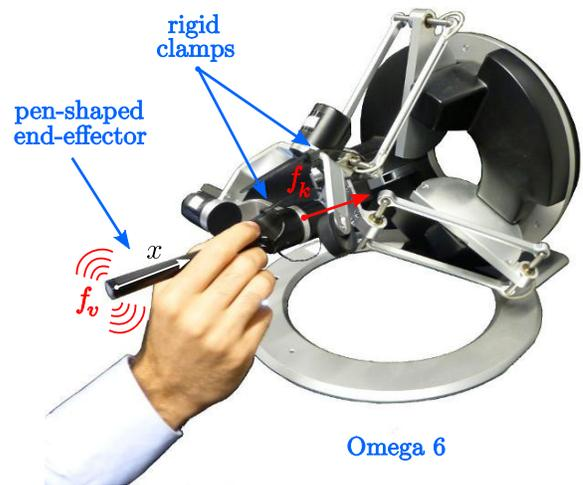
Fig. 4. Master system. The Omega 6 haptic interface enables the clinician to directly steer the needle while being provided with kinesthetic force  $f_k$  and vibratory force  $f_v$  about needle's ideal position and orientation, respectively. The motion of the haptic device is constrained along its  $x$ -axis.
