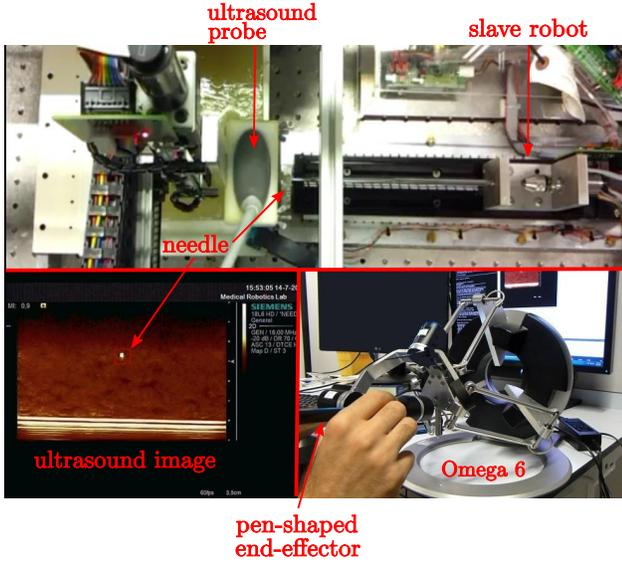
Fig. 5. Experimental test. The human operator, through the haptic device (bottom-right), steers the needle inside the soft-tissue phantom (top). The controller, through the ultrasound imaging system (bottom-left), tracks the needle and evaluates the ideal position and orientation of the needle tip to be fed back to the clinician via kinesthetic and vibratory force feedback. No visual feedback is provided.
