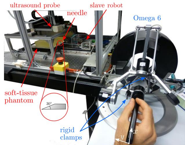
Fig. 1. Teleoperation system. The clinician, through the Omega 6 haptic device, controls the motion of the slave robot and, thus, the needle. The haptic interface also provides the clinician with navigation cues about the ideal position and orientation of the needle tip, evaluated by the steering algorithm.
