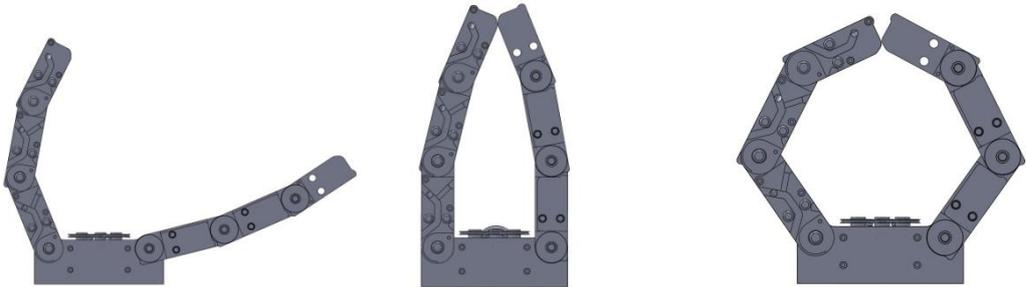
Figure 37: 3 different gestures that are possible with the 2-fingered hand design.
