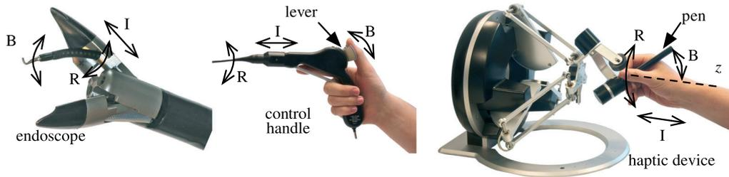
Figure 1. The Anubis endoscopic instruments have three degrees of freedom, insertion (I), rotation (R) and bending (B). For the conventional method, these are controlled by moving the control handle forwards and backwards (I), by rotating the control handle (R) and by using the bending lever (B). For the robotic method, these are controlled by moving the haptic device forwards and backwards (I), by rotating the pen around the z axis (R) and by rotating the pen away from the z axis (B)
