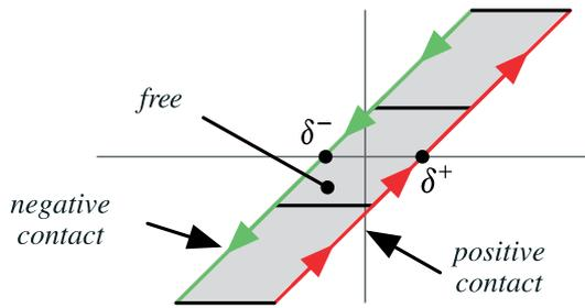
Figure 3. Hysteresis model: in the positive contact and negative contact modes, the instrument motion  $q$  follows the actuator motion  $c$ . In the free mode, the instrument is stationary
