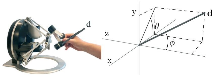
Figure 6. The direction of the pen of the haptic device ( $d$ ) controls the bending and rotation DOFs. The angle  $\phi$  controls the bending. The angle  $\theta$  controls the rotation
