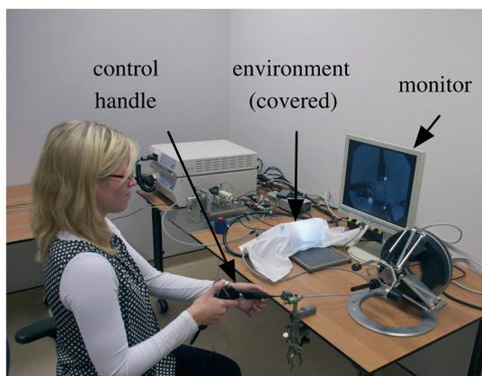
Figure 7. Subject performing the experiment using the conventional method under the endoscopic view condition
