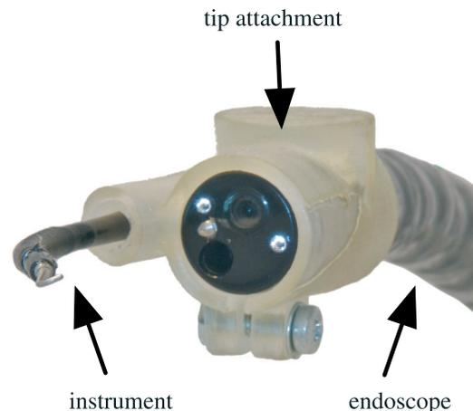
Figure 5. A tip attachment is fitted to the tip of the endoscope in order to guide the instrument
