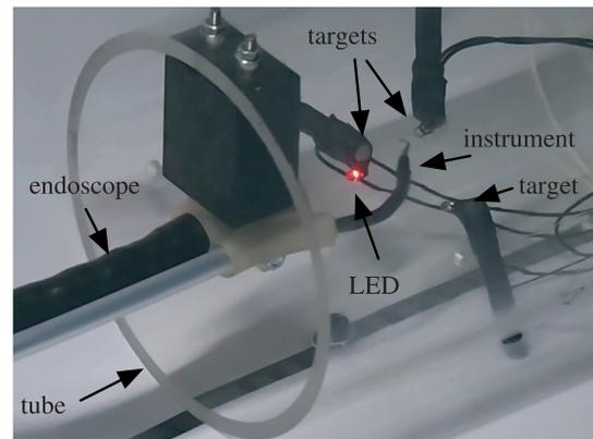
Figure 4. The environment for the experiment consisted of a transparent tube with three targets. The endoscope was fixed to the tube. LEDs were used to signal the subject which target was to be tapped
