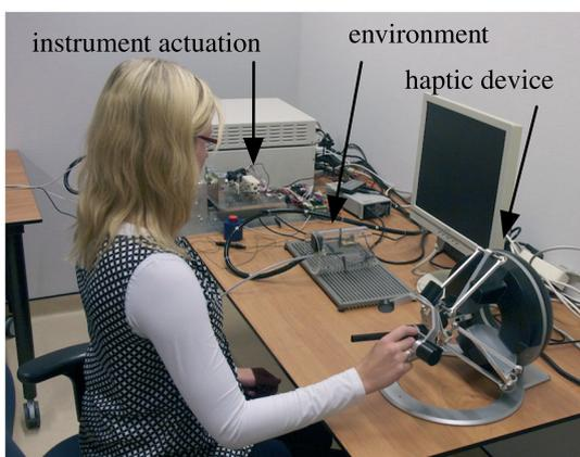
Figure 9. Subject performing the experiment using the robotic method under the direct view condition
