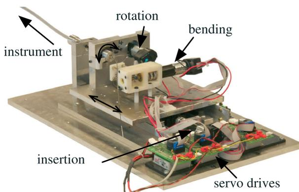
Figure 2. Actuation of the instrument: three motors actuate the insertion, rotation and bending DOFs of the instrument. The motors are controlled by servo-drives
