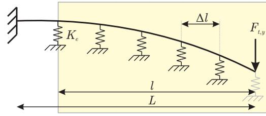
Fig. 3. The tissue elastically supports the needle as it is inserted into the tissue. This is modeled as a cantilever beam supported by a series of springs (with effective stiffness  $K_e$ ) along the needle shaft and  $F_{t,y}$  as the transverse tip force. The total needle length is  $L$  and the inserted needle length is  $l$ .
