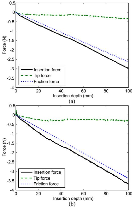
Fig. 10. The horizontal tip force ( $F_{t,x}$ ) is calculated by subtracting the horizontal component of the friction force ( $F_{f,x}$ ) from the insertion force ( $F_b$ ) for insertion at (a) 10 mm/s and (b) 20 mm/s.
