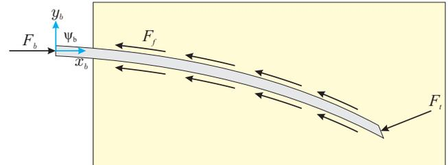
Fig. 1. As a bevel-tipped needle is inserted into a soft tissue, interaction forces are developed:  $F_b$  is the insertion force measured at the needle base,  $F_f$  is the friction force along the needle shaft and  $F_t$  is the force at the needle tip due to cutting of the tissue. The coordinate frame located at the base of the needle is indicated by  $\psi_b$ .
