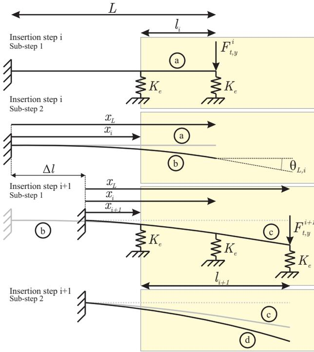
Fig. 4. Needle insertion into a tissue is modeled in a series of insertion steps. Each insertion step ( $i$ ) is divided into 2 sub-steps: in the first sub-step the inserted needle distance is increased with  $\Delta l$  and a spring of stiffness  $K_e$  is added. In the second sub-step, the deflected needle shape is calculated by applying transversal tip force  $F_{t,y}$ .
