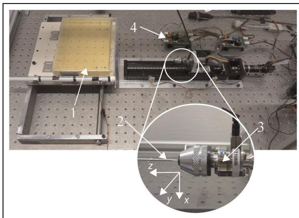
**Figure 1.** Two degree-of-freedom needle insertion setup used for the macroscopic observations. 1: Gelatin block; 2: needle; 3: force/torque sensor; 4: controllers. Insertion is along the  $z$ -axis, and the needle is oriented such that deflection is predominantly in the  $yz$ -plane.
