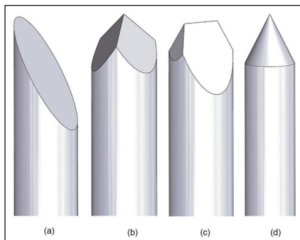
**Figure 2.** Various needle tip shapes used in the experiments: (a) bevel, (b) franseen, (c) diamond, (d) conical.
