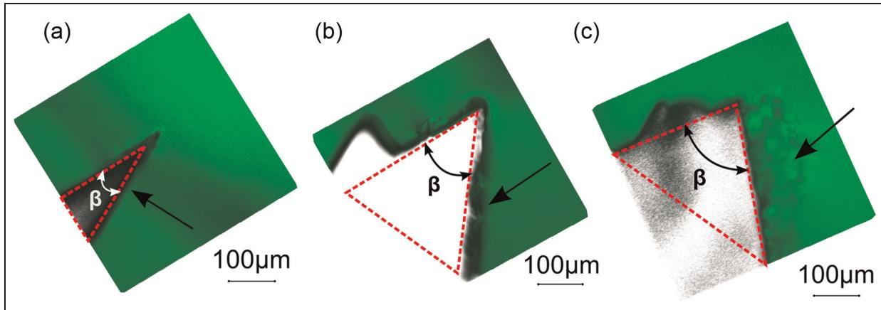
**Figure 8.** Epifluorescent images of gel compression (shown with an arrow) for variation in bevel angle ( $\beta$ ): (a)  $30^\circ$ , (b)  $60^\circ$  and (c)  $75^\circ$ . Compression is observed to be most for  $\beta = 75^\circ$ .
