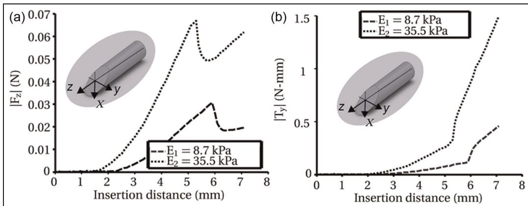
**Figure 12.** Variation in insertion force ( $|F_z|$ ) and in-plane bending torque ( $|T_y|$ ) for change in gel elasticity ( $E_1$  and  $E_2$ ). The needle diameter ( $\phi$ ) and bevel angle ( $\beta$ ) are 1 mm and  $60^\circ$ , respectively. The needle is inserted at  $v = 0.5$  mm/s.
