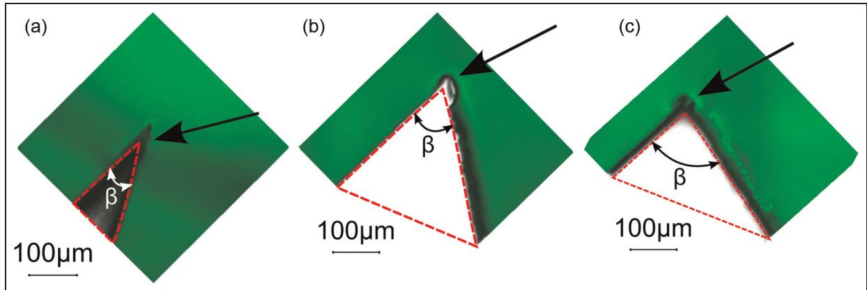
**Figure 7.** Epifluorescent images of gel rupture (shown with an arrow) for variation in bevel angle ( $\beta$ ): (a)  $30^\circ$ , (b)  $60^\circ$  and (c)  $75^\circ$ . Rupture is observed to be longest and narrowest for  $\beta = 30^\circ$ , while it is shortest and widest for  $\beta = 75^\circ$ .
