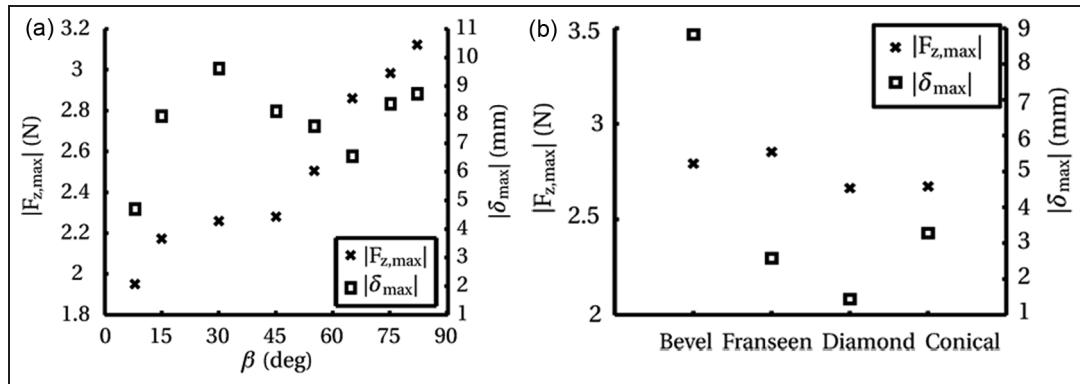
**Figure 5.** Maximum insertion force  $|F_{z,\max}|$  and maximum needle tip deflection  $|\delta_{\max}|$  for variation in: (a) bevel angle ( $\beta$ ) and (b) tip shape. In both experiments,  $E_2=35.5$  kPa,  $v=10$  mm/s and  $\phi=1$  mm. Average standard deviations in (a) for  $|F_{z,\max}|$  and  $|\delta_{\max}|$  are 0.08 N and 0.15 mm, respectively. Average standard deviations in (b) for  $|F_{z,\max}|$  and  $|\delta_{\max}|$  are 0.14 N and 0.18 mm, respectively.
