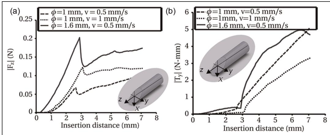
**Figure 11.** Variation in insertion force ( $|F_z|$ ) and in-plane bending torque ( $|T_y|$ ) for changes in needle diameter ( $\phi$ ) and insertion velocity ( $v$ ). The bevel angle ( $\beta$ ) is  $30^\circ$ . The needle is inserted into the gel of elasticity  $E_2 = 35.5$  kPa.
