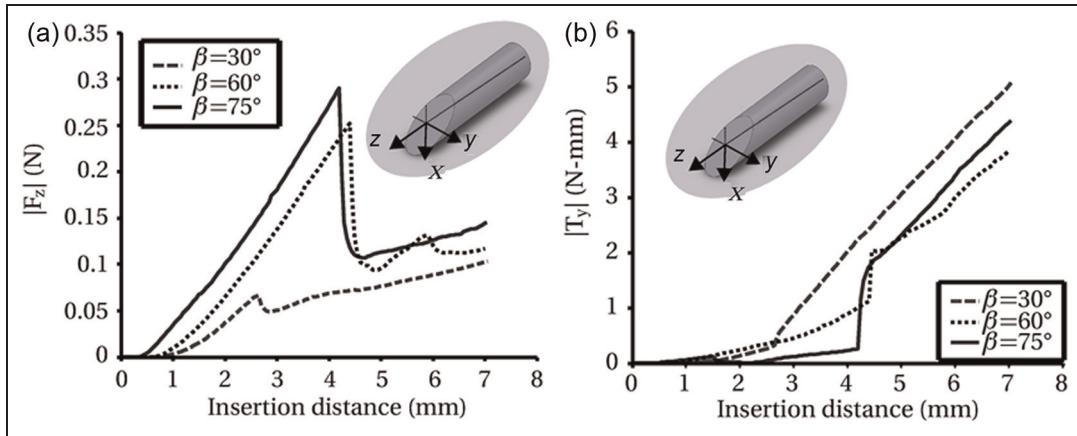
**Figure 10.** Variation in insertion force ( $|F_z|$ ) and in-plane bending torque ( $|T_y|$ ) for change in bevel angle ( $\beta$ ). The needle diameter ( $\phi$ ) is 1 mm. The needle is inserted at  $v = 0.5$  mm/s into a gel of elasticity  $E_2 = 35.5$  kPa..
