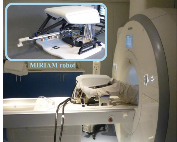
Fig. 1 The MIRIAM (Minimally Invasive Robotics In An MRI environment) robot is a 9 degrees-of-freedom magnetic resonance (MR)-compatible system designed for transperineal prostate biopsy. The system is capable of inserting, rotating and firing a biopsy needle to collect tissue samples.
