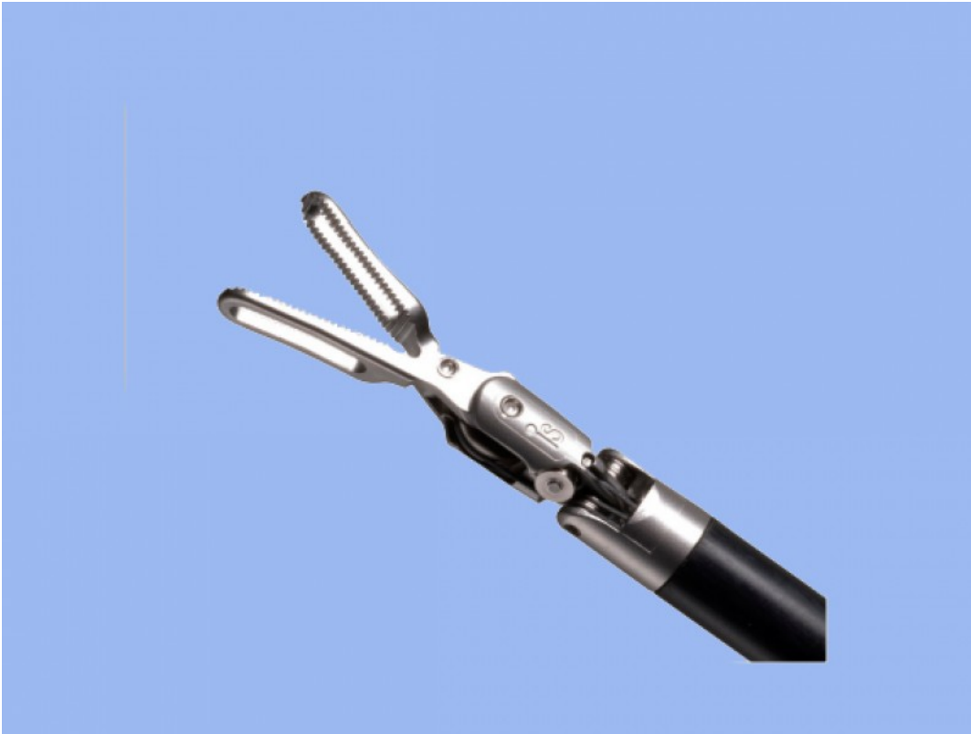
Figure 2.2: The tip of a Da Vinci robot tool with two hinges
