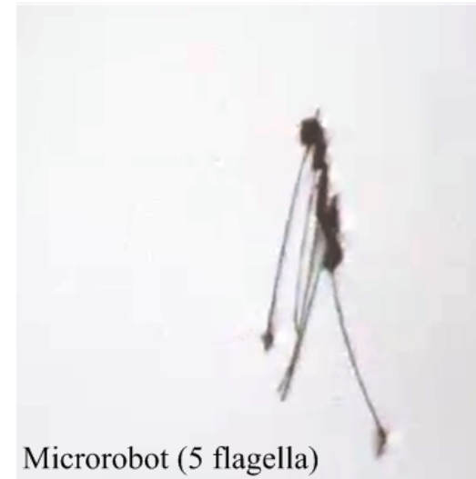
FIGURE : Soft microrobots with multiple flexible flagella
