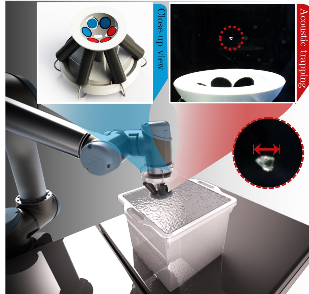
A robot arm carries acoustically-powered device which can trap and maneuver particles underwater
