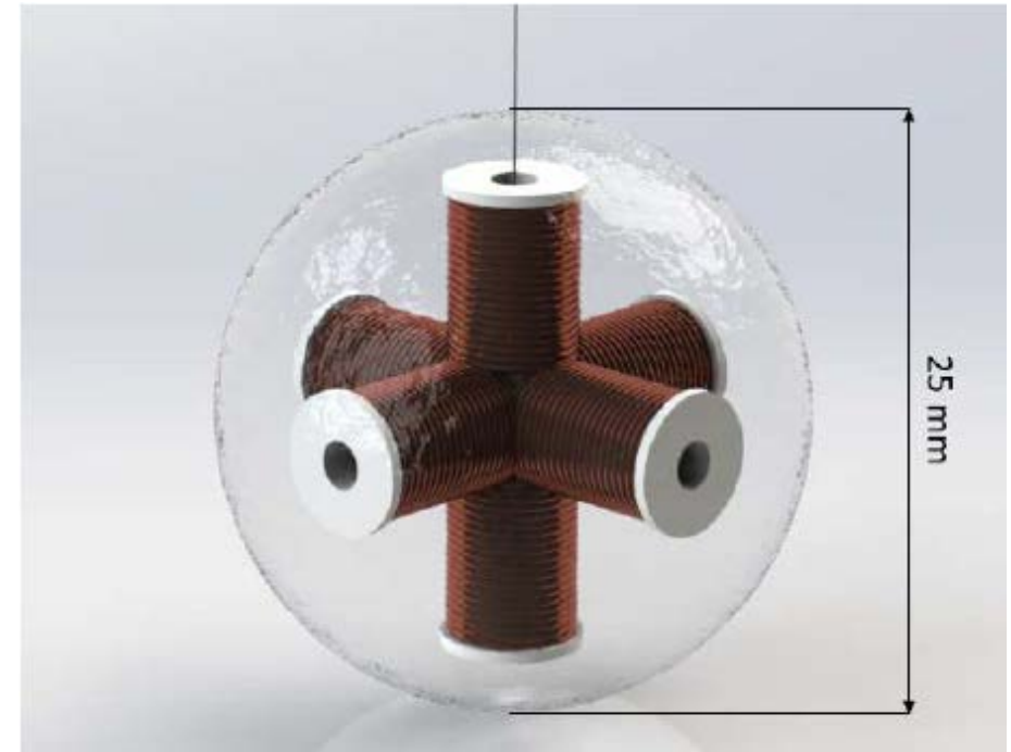
FIGURE : A miniature tri-axial electromagnetic coil will generate a controlled magnetic moment and its dipole will align along external magnetic fields.
