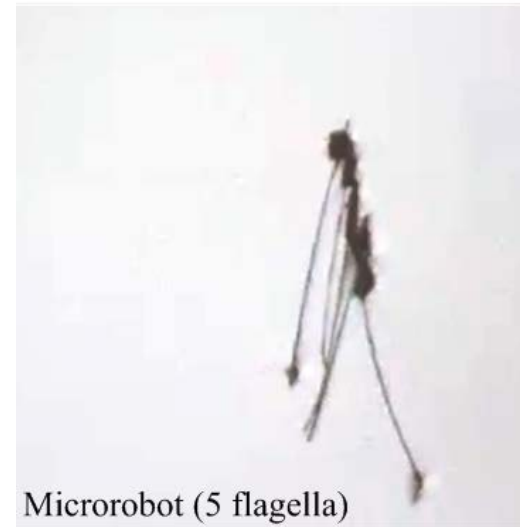
FIGURE : Soft microrobots with multiple flexible flagella
