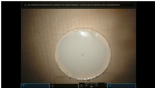
FIGURE 5.9: Phantoms 2: Spherical agar-agar phantom in white light The ICG was dissolved in PBS and buried 2.4 cm below the surface of the phantom.
