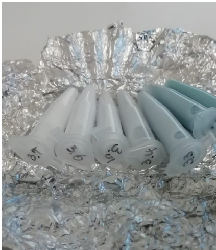
FIGURE 5.13: Phantoms 3: The eventual phantom This figure shows the eventual phantom and the five different concentrations of ICG used for the measurements.
