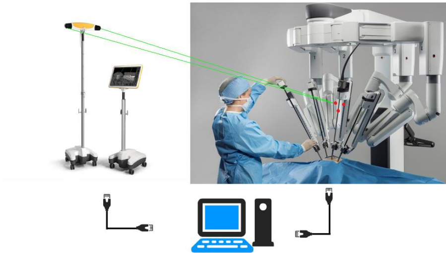
Figure 1: A visual representation of the proposed design. Left: the conventional Brainlab navigation system registers the IR markers on the Da Vinci stereo camera (right). Below: a computer runs an application that combines information from Brainlab and the video feed from the camera.
