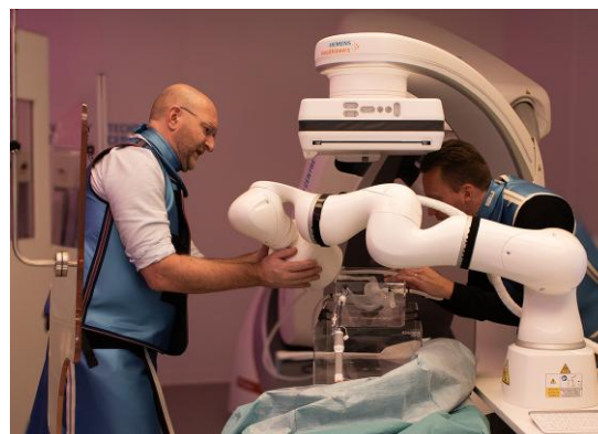
Figure 2 A pre-clinical magnetic actuation system by Flux Robotics B.V., comprising of a robot arm and electromagnet. A surgeon (left) steers a magnetic guidewire in an aortic phantom by hand-guiding the Flux One™ robot and manipulating the electrical current through the electromagnet, during a simulated fenestrated endovascular aortic aneurysm repair (f-EVAR) intervention
