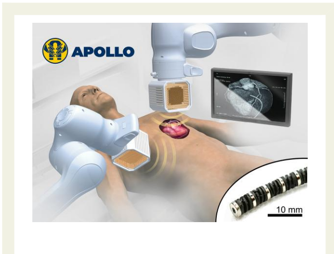
Figure 1 APOLLO concept: a collection of robotically positioned magnets ex vivo accurately steer a magnetically actuated probe to the target location in vivo . An experimental probe design is shown in the bottom right corner, comprising multiple interacting permanent magnets and magnetic polymers. 7 APOLLO will develop robust hardware and software to guide dextrous probes for minimally invasive endovascular interventions
