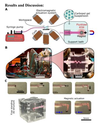
**A.** MagNoFE3D embedded printing system consisting of an injecting syringe pump and an electromagnetic system to steer the plotting magnet. The movement of the magnet locally fluidizes the Carbopol support bath, opening space and guiding the ink. **B.** Picture of the experimental setup and a double helix printed with coloured water. **C.** Printing, photocuring, washing and actuation of a 3D structure using a photocurable ink.
