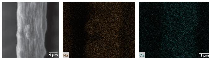
Figure 5.S4: Zoomed-in scanning electron microscopy (SEM) image on the tail of a tadpole-like microrobot and energy-dispersive X-ray spectroscopy (EDS) elemental mapping images of Na and Ca.
