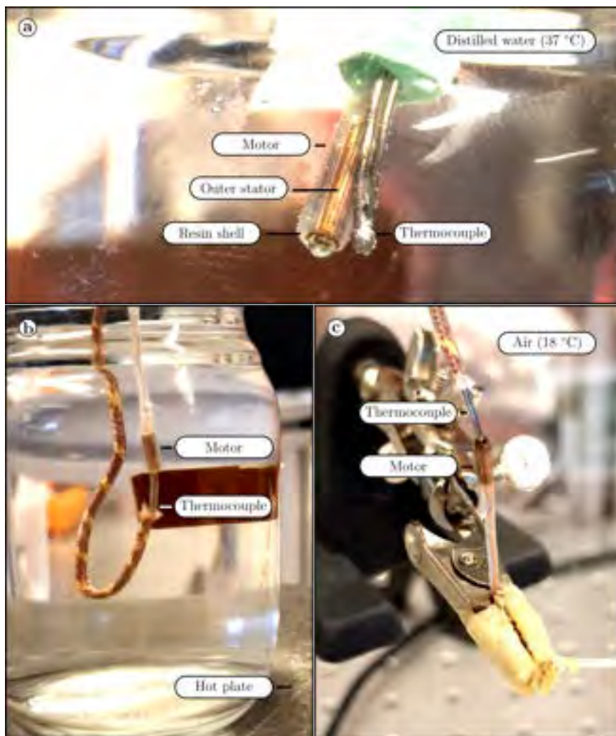
Figure S6.3: Temperature measurements. a External temperature measurement inside a bath of distilled water at 37 °C. Visible are the motor with outer stator and resin shell, but without the permanent magnet rotor, and a thermocouple placed along its outer surface. b Internal temperature measurement inside a bath (glass jar) of distilled water at 37 °C. The thermocouple is placed inside the motor's rotor cavity. The water is heated with a hot plate. c Internal temperature measurement inside air at 18 °C.
