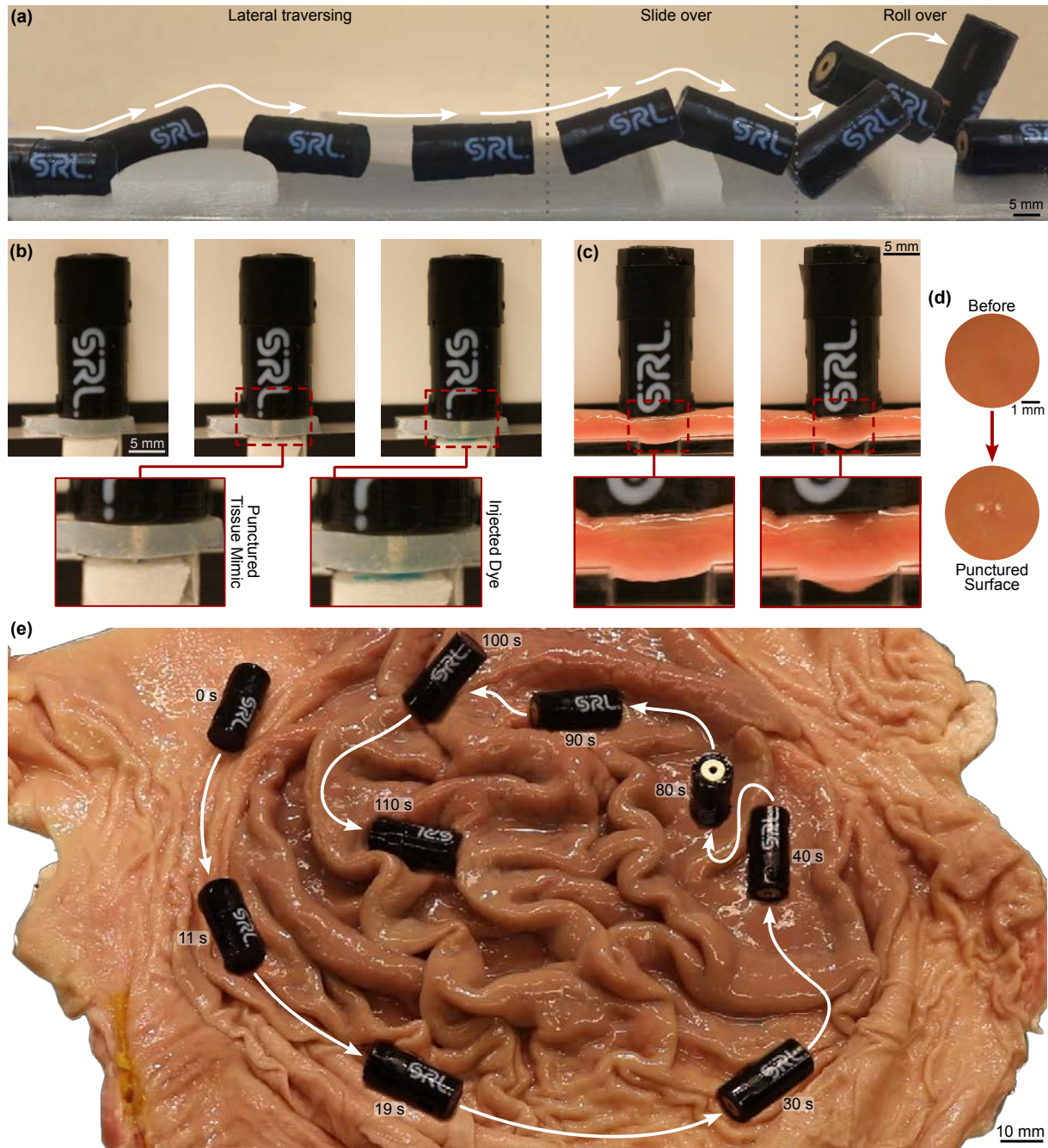
Fig. 5 Demonstration of targeted needle-based drug delivery and navigation. a) Locomotion strategy of the capsule robot can be adapted to different types of obstacles encountered during navigation. Please refer to Supplementary Movie 3 for demonstration of the locomotion capabilities. b) Contactless inductively triggered puncture and dye injection into a soft tissue mimic. Please refer to Supplementary Movie 4 for a complete demonstration. c) Contactless inductively triggered puncture into ex vivo porcine stomach tissue. Please refer to Supplementary Movie 5 for demonstration of the ex vivo capabilities of the capsule. d) Tissue surface before and after puncture, showing the penetration mark created by the needle. e) Magnetic navigation of the capsule robot along a spiral trajectory on the inner surface of a porcine stomach.
