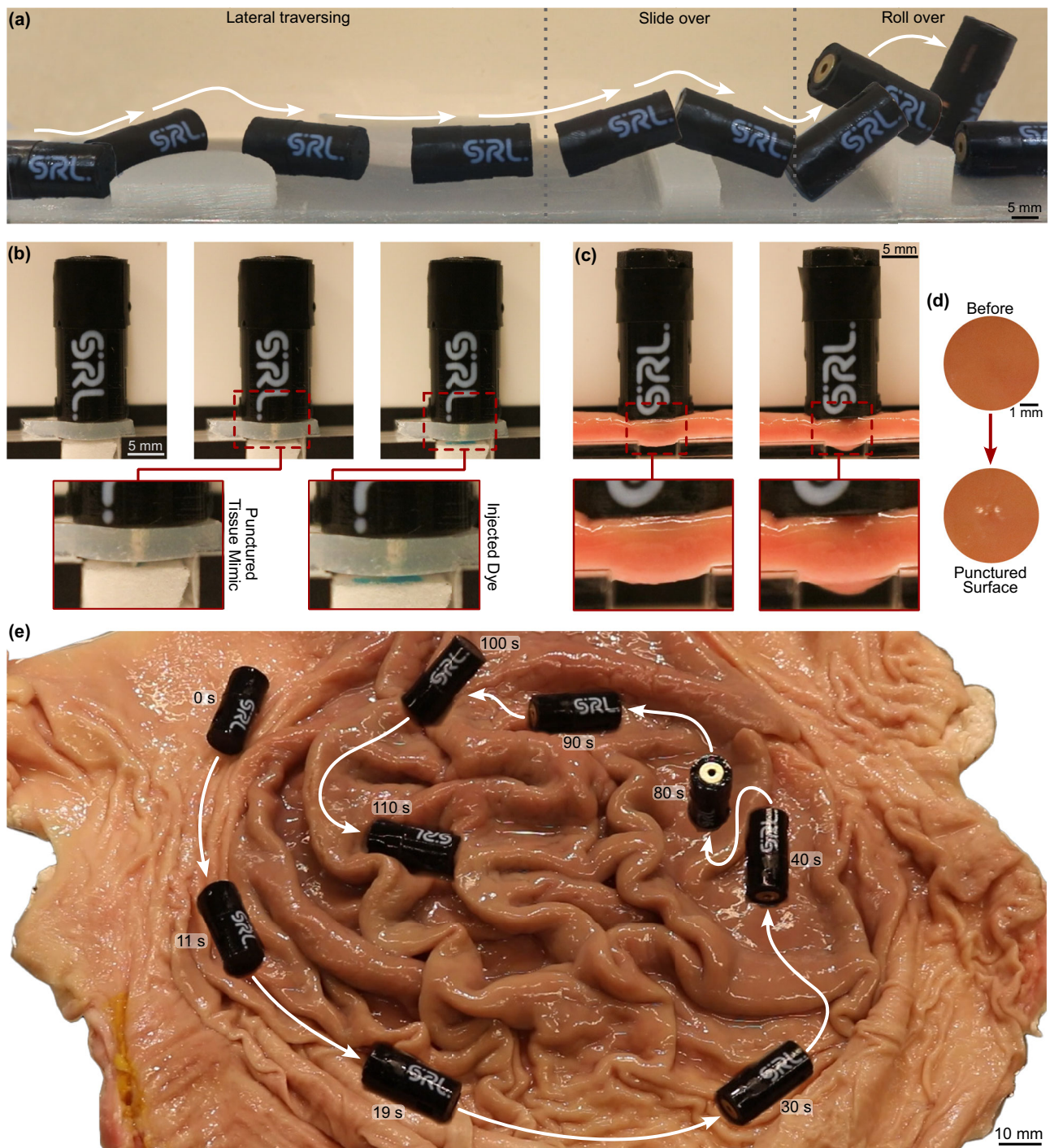
Fig. 5 | Demonstration of targeted needle-based drug delivery and navigation. a Locomotion strategy of the capsule robot can be adapted to different types of obstacles encountered during navigation. Please refer to Supplementary Movie 3 for demonstration of the locomotion capabilities. b Contactless inductively triggered puncture and dye injection into a soft tissue mimic. Please refer to Supplementary Movie 4 for a complete demonstration. c Contactless inductively triggered puncture
